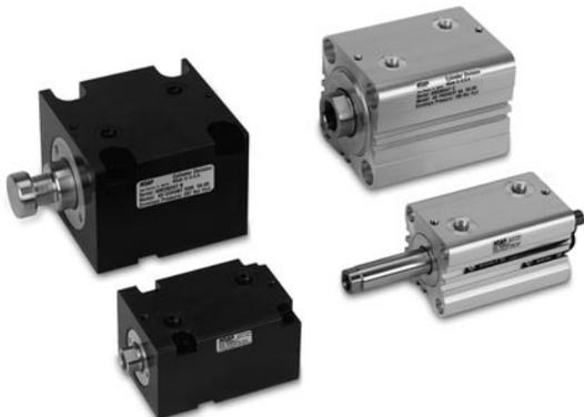
Series CHE aluminum compact hydraulic cylinders are available with magnetic piston option for position sensing and for up to 140 BAR operating pressure. Series CHD steel compact hydraulic cylinders are available for up to 207 BAR operating pressure.
